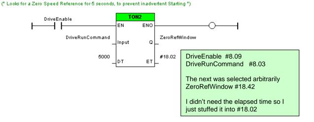
The final bit of logic is the actual Zero Reference Start logic.
