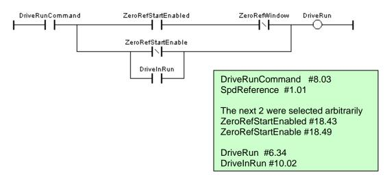
If the **DriveRunCommand** is ascerted **AND** the **ZeroRefStartEnable** bit is **not ON**, then the drive works normally as it would out of the box.
